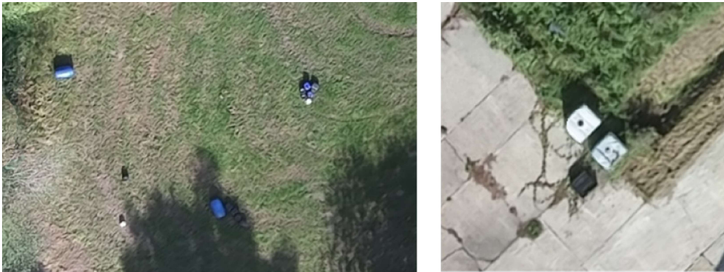
Figure 5.4. Drone images of objects tested for detection with DL algorithms: several barrels and jerrycans on the left and two IBCs on the right. Source: The authors in collaboration with Belgian federal Police.
