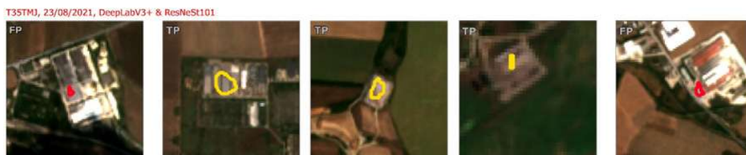
Figure 4.6. Inference results on different dates from a Sentinel-2 tile in Romania, showing false positive (red) and true positive results (yellow). Source: The author.
