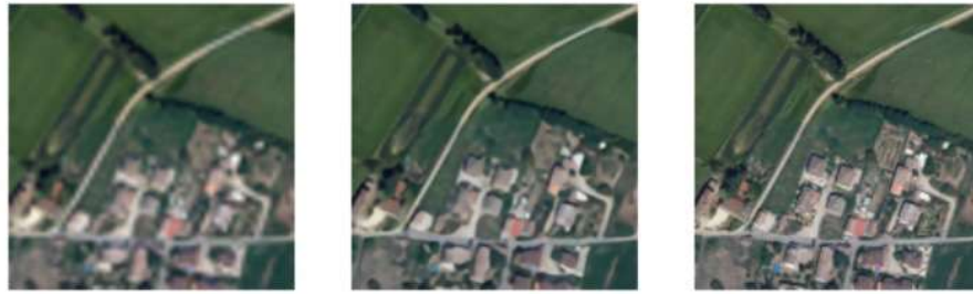
Figure 4.3. Examples of images (from left to right) showing our SR enhancement: the input image, before SR enhancement (low resolution), the output image (following SR enhancement) and the ground-truth (HR) image. Source: The author.
