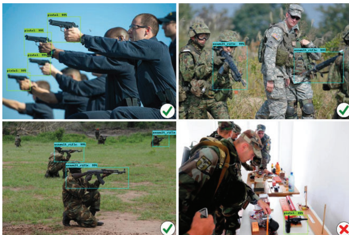
Figure 2: Results obtained from the test image data set. Top: All weapons have been correctly detected and annotated by the 2-pass object detector. Bottom left: All but one assault rifle have been correctly detected and annotated. Bottom right: Combination of two objects mistakenly classified as pistol.
